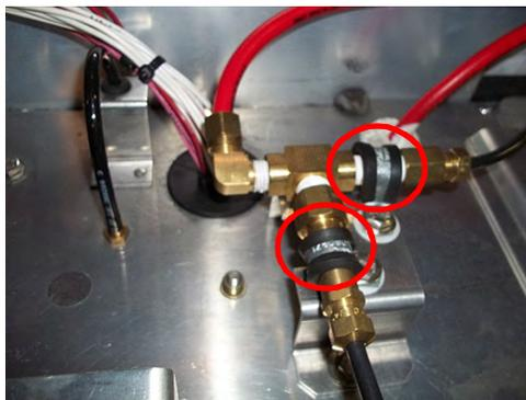
Figure 5.6 Clapets anti-retour
