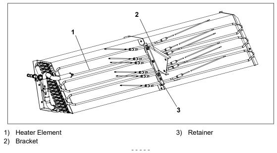
The heaters are wired directly back to the contactor and if a heater failure occurs during a trip, the heater set containing that heater may be disconnected at the contactor.
