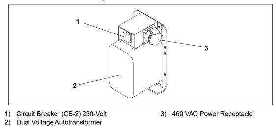
Figure 7.20 Autotransformer
