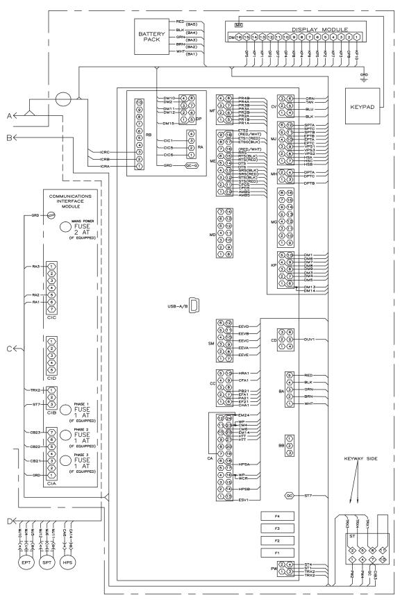
Figure 8.4 Unit Wiring Diagram (Sheet 2 of 2)
