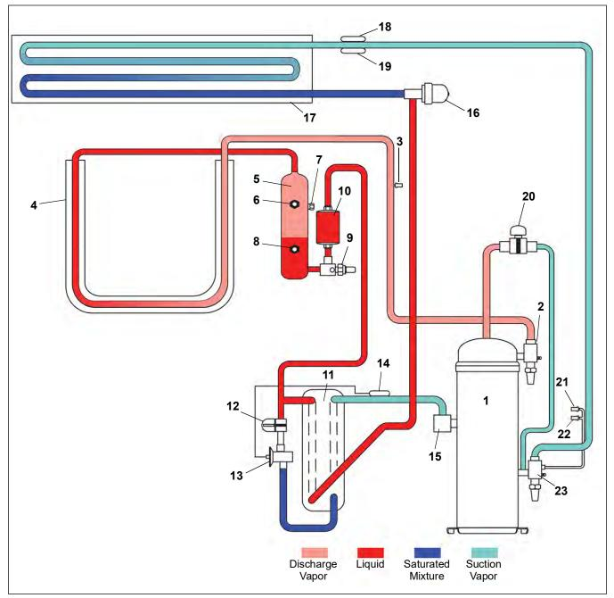
Figure 3.8 Refrigeration Circuit Schematic - Economized Operation
