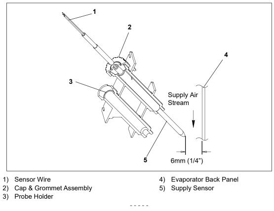
Figure 7.34 Supply Sensor Positioning
