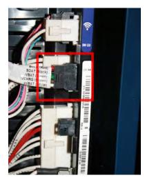
4. Using a Driver Bit, Carrier Transicold part number 07-00418-00, loosen the left hand screw on the battery pack cover then remove the second screw on the outer edge of the battery pack cover.
