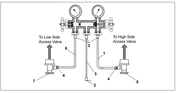
Figure 7.2 Manifold Gauge/Hose Set
