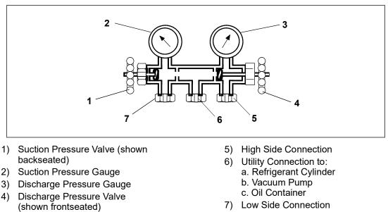
Figure 7.1 Manifold Gauge Set
