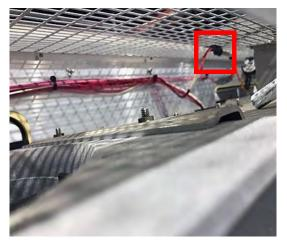
4. Cut all the wire ties (see Figure 7.25) that are securing the sensors to the harness and remove sensor.
