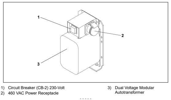
Figure 5.1 Autotransformer
