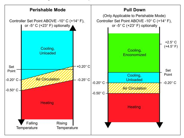
Figure 4.4 Controller Operation - Perishable Mode
