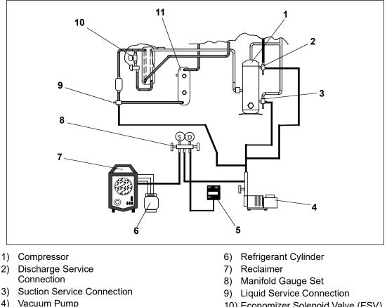
Figure 7.4 Refrigeration System Service Connections
