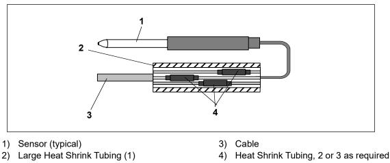
Figure 7.33 Sensor and Cable Splice
