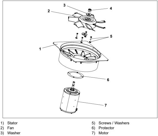
Figure 7.11 Evaporator Fan Assembly
