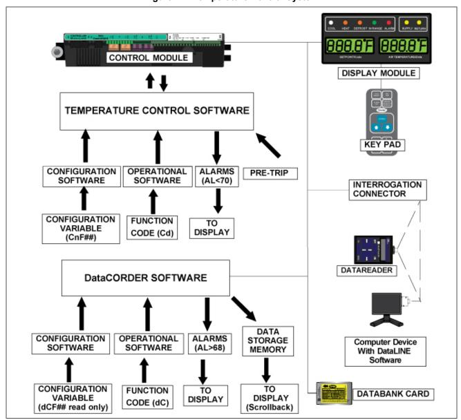
Figure 4.1 Temperature Control System
