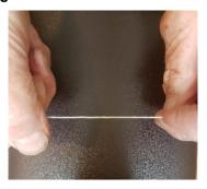
Figure 7.10 Loctite 55 - Locate Threads
