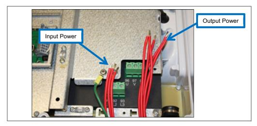
6. Cut the barrels off of the wires using wire cutters and strip back the insulation approximately 0.25" (6.35mm).
