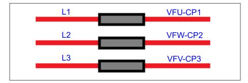
8. Position the heat shrink and crimp the electrical splice connector for all 6 wires mentioned above.
