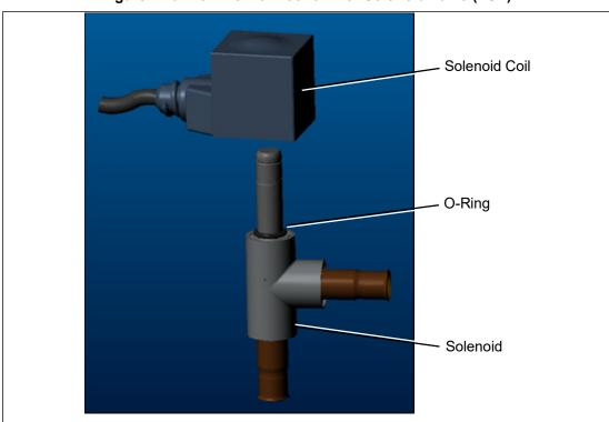
Figure 7.19 Coil View of Economizer Solenoid Valve (ESV)
