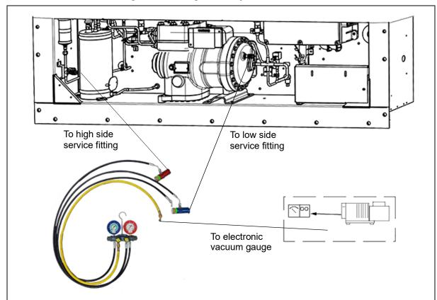
Figure 7.2 Refrigeration System Evacuation
