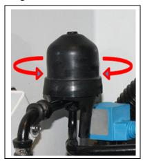
Figure 7.18 HPXV Valve Body Dimples
