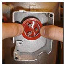
Figure 7.8 Installing Orange Gasket
