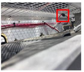
Figure 7.25 Return Sensors - Bracket
