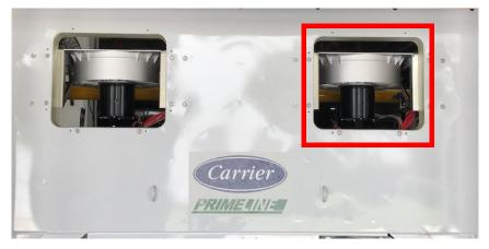
Figure 7.24 Removing Evaporator Motor
