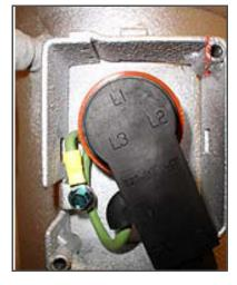
19. Connect the green ground wire (Figure 7.10 above) to the grounding tab located inside the terminal box of the compressor using the self tapping grounding screw (Figure 7.5, item #12). Close the compressor terminal box using the terminal cover removed.
