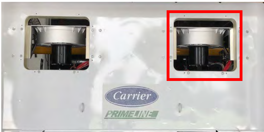
Figure 7.22 Removing Evaporator Motor
