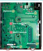
**Pic 2.** If possible leave the black safety cover on. The two screws at center should never be removed.
