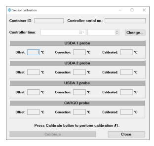
When placing the USDA and cargo probes in ice water, they should display 0°C. If any reading deviates from this value the probe requires calibration. Calibration is simply done by looking at the reading for the USDA sensor and then double clicks in e.g. CalUs1. In the popup window enter the calibration value required in order for the sensor to reach 0°C. Then press Calibrate.
