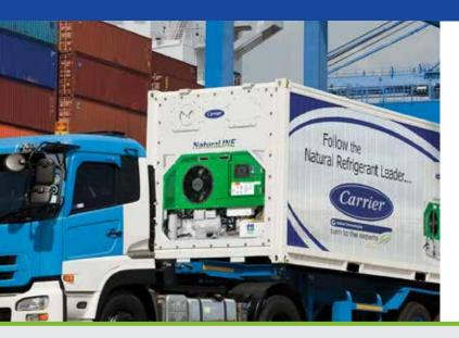
Natural refrigerant technology responds to the shipping industry's drive for sustainable refrigerated transport solutions. Among all the natural refrigerant alternatives, none presents a better solution for shipping lines than carbon dioxide (CO<sub>2</sub>), which is used in the NaturaLINE® container refrigeration system from Carrier Transicold.
